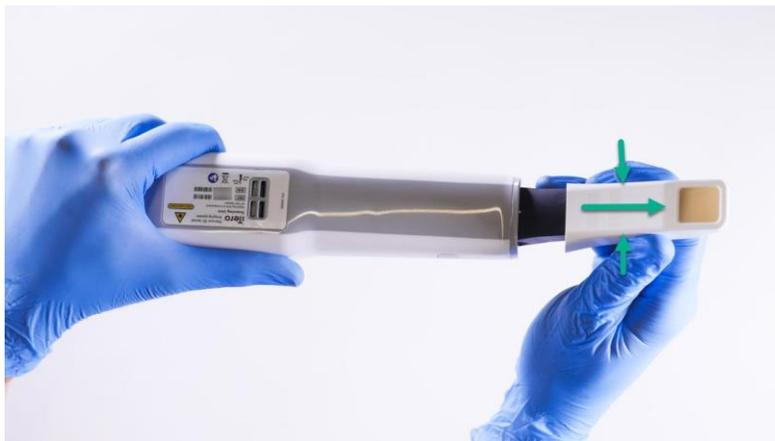
Figure 8: Removing a wand sleeve
